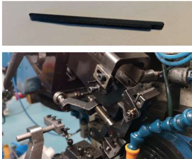
Figure 27: 3D printed separator finger
