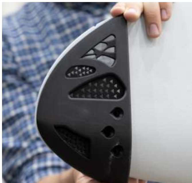
Figure 34: Composite prototype of lightning tip receptor
