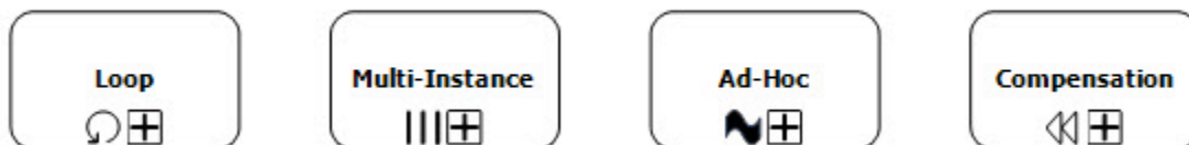
Figure 11- Loop, Multiple instances, Ad-hoc and Compensation
