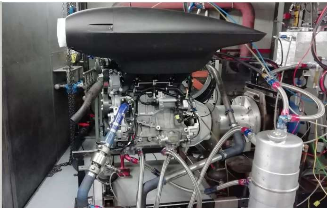
Figure 30: 3D printed Airbox
